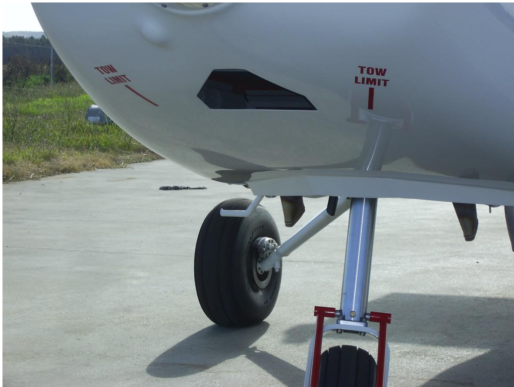
Figure 1 – Tow Limit Markings on Lower Engine Cowl
