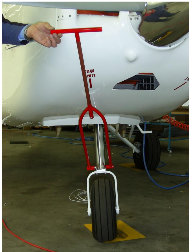
Figure 2 – Tow Limit Markings Tolerance Check
